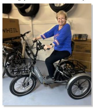
eBikes. It's foldable with a battery that will last from 4-6 hours on a charge. The top speed is 14 mph with five levels of pedal assist.
