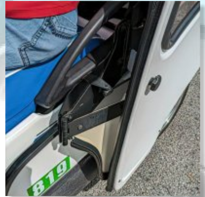
The doors are self-closing, and the cart can be driven with them open or closed.
